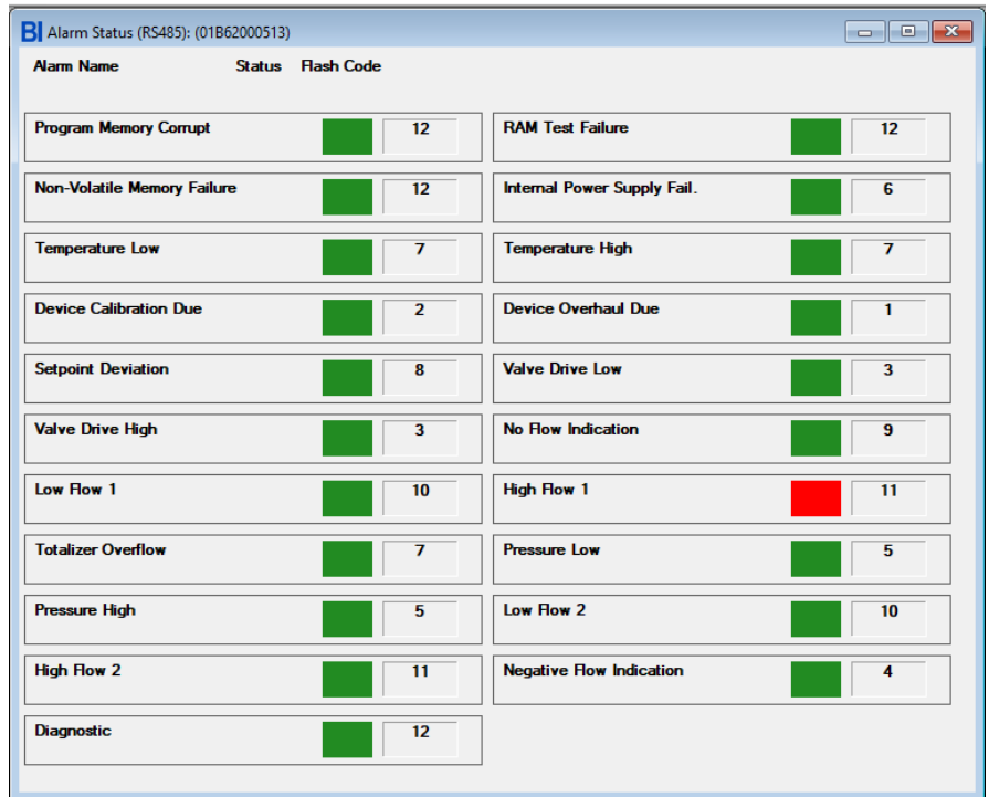
Figure 8-4 Alarm Status Window (RS485) (Actual alarms may vary depending upon device type)
