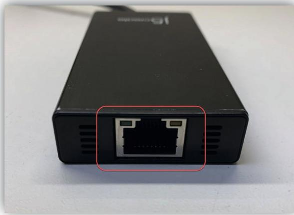
Once the PC settings have been changed and the cable is physically connected between the PC adapter and the BCU, open a web browser and enter the IP address of the BCU (default 192.168.1.100) as the URL at the top. Hit “Enter” or click “Go” to load the BCU Embedded Web Interface.
