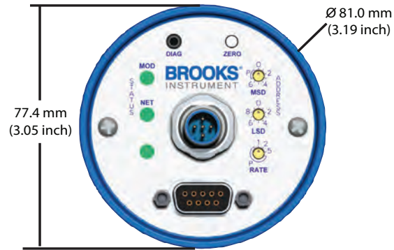
Figure 17: DeviceNet Top Dimension
