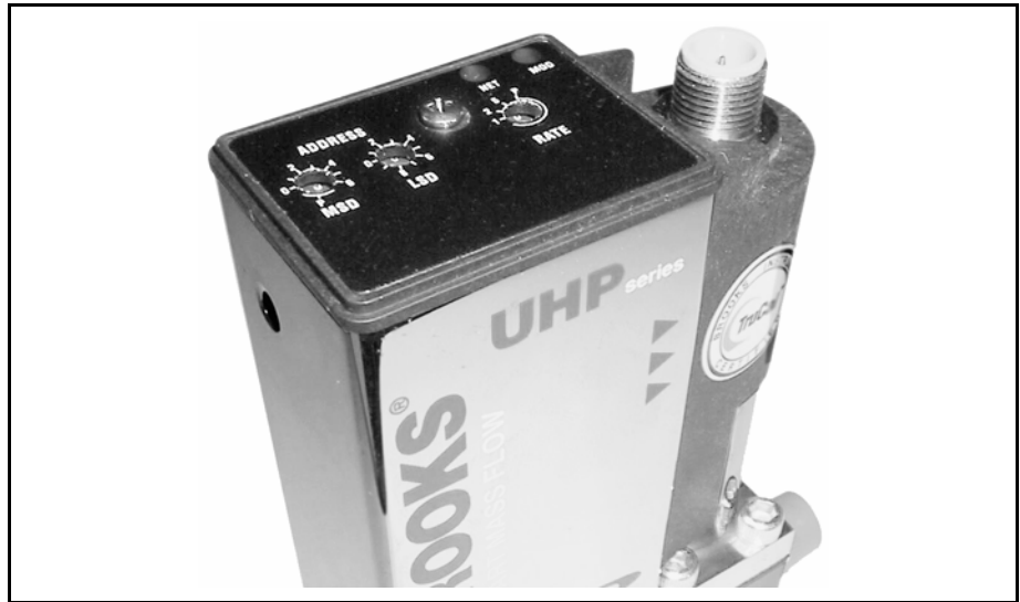
Figure 3-4 View Showing Top of PC/PM Can
